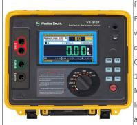
The VS-3127 **5kV Insulation Tester** offers the ability to perform accurate insulation resistance measurements up to 15 kV test voltage with a maximum resistance of 30 T $\Omega$ . Resistance measurement accuracy is  $\pm$  5 % from 1 M $\Omega$  to 3 T $\Omega$ !
